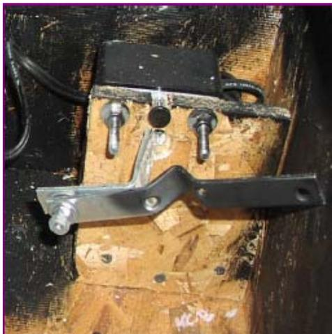
We had to make the bracket for the motor ourselves. It is simply (1) L-shaped bracket, filed down on one end to fit inside the shaft of the rotisserie motor, and (1) flat metal mounting plate, cut to the appropriate length and bent in the middle. (See photo).
