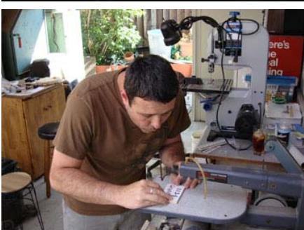
Time for the lettering. I wanted the finished plaque to look like it was a bronze casting. I felt I couldn't achieve this with carving only the foam. I made the decision to cut out each letter from 1/4 inch hobby plywood with a scroll saw. By doing this I made sure that all the lettering had crisp edges.
