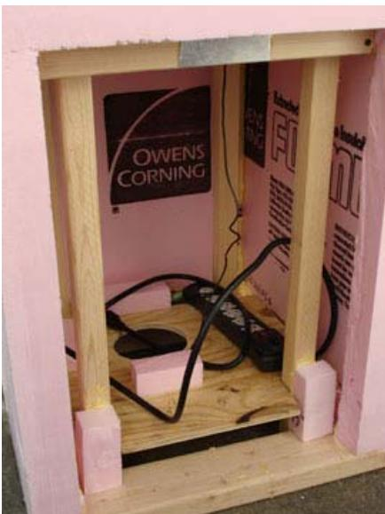
I left one sheet of foam off of the bottom so that I could have access to the bottom space. Later I added a sub woofer and power strip in this space. When most of the foam was glued and in place, it was time to start shaping it up. I used a free form hot wire cutter to remove large chunks out of the foam to create the angle.
