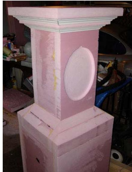
I used sand paper to start refining the shape, clean up the angle and remove some of the excess glue. After that I used PVC crown molding to cheat the details around the top. I set them in place with hot glue. The opening for the plaque was engraved into the foam using a wood router.
