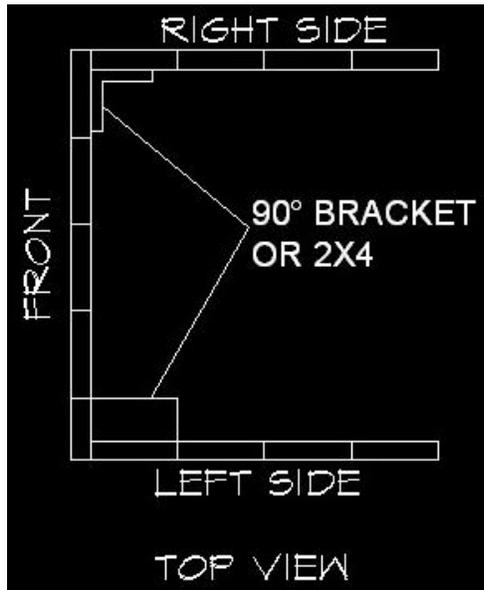
Take the 3 sides we just built and get either a 90 degree bracket or a 2x4 and screw it the very edge of the front of one of the sides. We want the front side of the box to overlap the sides. Now get the front and make the edge of that even with the edge of the side. Do the same on the other side. If you use the 90 degree brackets, you can put 2 on each corner but make sure the top one is at the very top so it will not hit the pipe, and if you use a 2x4, put it right in the middle.
