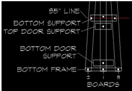
Now cut another 1x4 and screw this one right under the one we just did. This board is going to be the Top Door Support. Make sure this board does not go under the two outside boards. Those boards are not part of the door. Get another 1x4 and cut to size right above the bottom frame board, this will be the Bottom Door Support. Again, do not let these go under the two outside boards. Make sure your screws are in the right place, as shown in the picture to the right.
