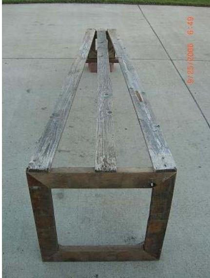
Put the 2' square on it's side on the ground and then get the 1' square and make it 6" off the ground. I used a brick and a 2x4 (you can see it in the picture a little bit). Get an 8' 1x4 (part of the free fence I found on the side of the road) and screw it to both the top and bottom pieces. Now put the edge pieces on and make these tilt inward at the top. Screw them down and do this on the two sides that touches this side. Leave the front side open because we will need that open for later.
