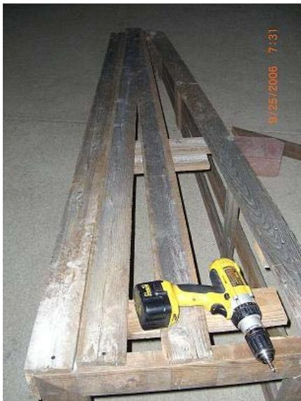
After you have screwed on the support boards, the door support boards, and the pipes, it is now time to start filling it in. Get another 1x4 and lay it down on the inside of the outside boards. Let this board tilt in the same like the two outside boards.
