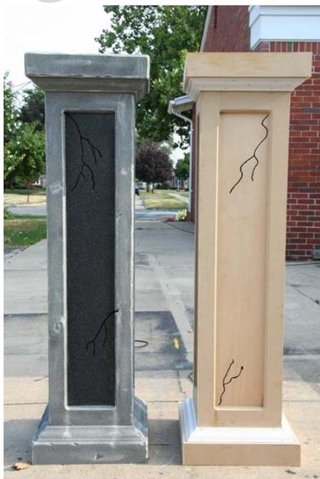
The big difference is cutting into the wood and making it look old. You can also see the inside edges are decorative. This is easily done with a router and the wood holds the detail.
