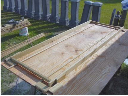
Here the jig is loaded with the first four panel pieces.
