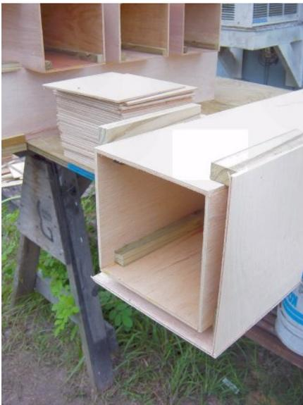
In keeping with the overlapping square method, spacer blocks are nailed at each corner of the center column. Bulking this section out in wood serves two purposes for me. It's slightly faster than adding third or fourth layers of sheet foam (3/4" styrofoam is our maximum available thickness around here.)
