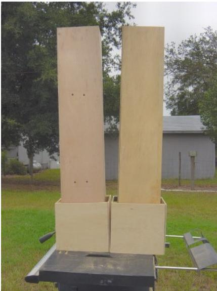
So far with this build, everything has been built square. Building square simplifies most of the process, as most machines are designed to cut straight lines, square, or parallel lines. Square assemblies require less intricate layout work, less time orienting components, and less opportunity for error when assembling multiple pieces at once.
