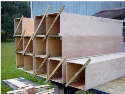
After adding the final side, check the assembly for square. Scrap wood can be nailed across corners to maintain square while the glue cures.
