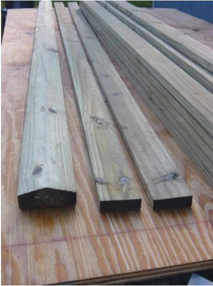
Basic sawing operations are required to prepare the dimensional pressure treated lumber.
