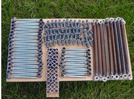
This is the fabricated hardware needed to build twelve fence posts.
