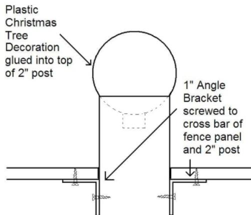
Screw angle brackets to the end of each fence cross bar.
