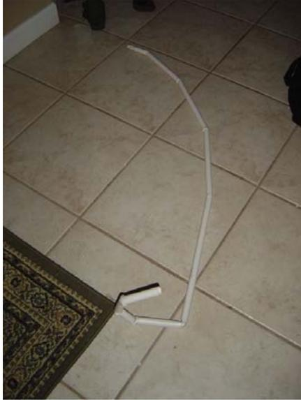
I started with a 5 foot section of 1/2 inch PVC and used the heat gun to bend the bottom into a circle, and the rest of it into a curved "stem".
