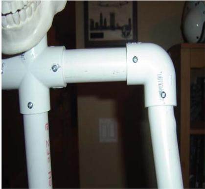
I also used the heat gun to bend the arms some. The 90 degree fitting was not letting the arm go outward enough, and the 45 degree one was TOO far.
