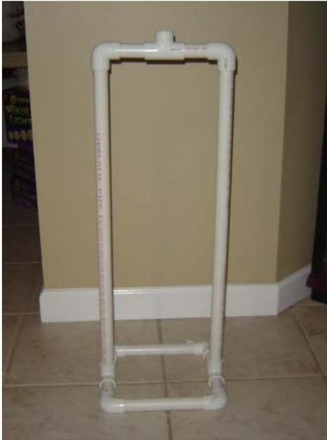
I started with a square base using 90 degree fittings and then built up with legs to the hip section, making sure everything was square and level.
