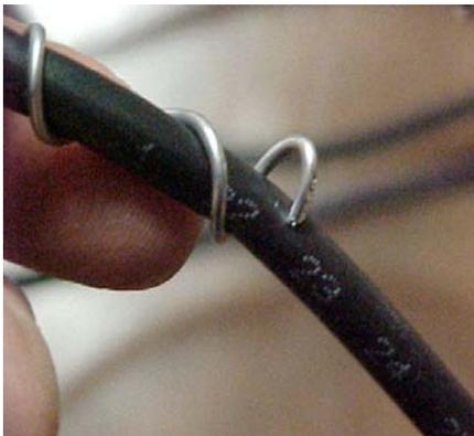
Now I'm taking a minute to push all the sharp ends of wire into the tubing. This will keep your skin in tack and make your prop safe. What I do is bend the wire so the sharp end is pointed into the tubing. Then using your long nose pliers just push the wire thru the tubing. This also makes the frame stronger.
