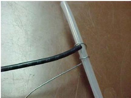
I put the 4" of wire from one end thru the hole I drilled in the back bone as in the picture here. Then I wrapped the wire around the back bone twice as in the picture.
