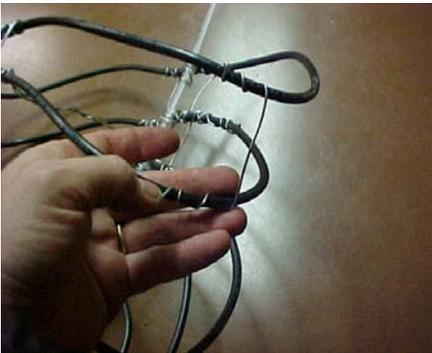
Now I'm adding supports between the ribs. I just wrap a wire around one rib than wrap the other end around the rib under it. Look at the picture below to see how I placed the rib supports.
