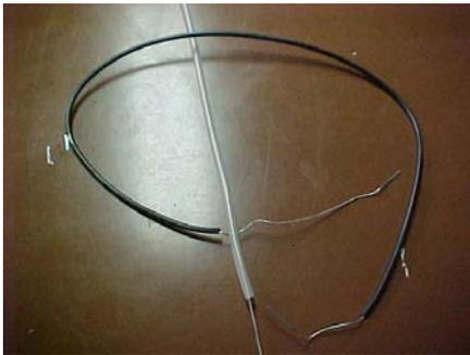
Now insert the wire in the tubing leaving 4" of wire sticking out of each end of the tubing. I will use the 4" of wire at each end to connect the rib to the back bone.
