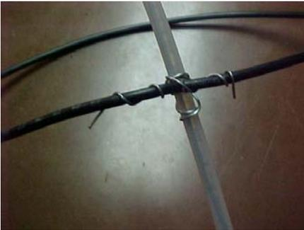
Now as you can see in the middle picture I now take the wire that's wrapped around the back bone and wrap it around the ribs. Take a minute and look at the pictures. This will secure the rib to the back bone. Don't worry if it feels loose because this is just building the basic shape. Later I will use more wire to make everything stronger.
