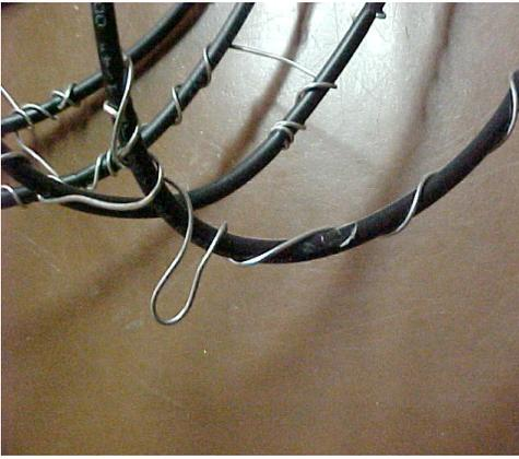
In the two pictures above I have added the loops that the arms connect to. I just wrap some wire around the rib were I want to attach the arms to.
