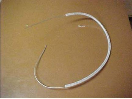
Now insert the wire in the tubing leaving 8" sticking out one end and 10" out the other end.
