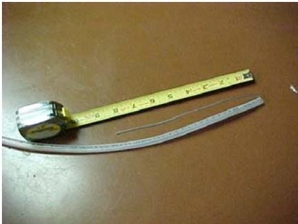
The first thing I do is cut a 24" long piece of 3/8" tubing and a 46" pieces of 12 gauge wire.
