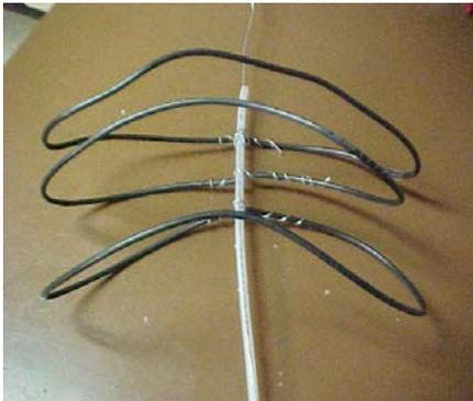
I have to make 4 more ribs so I will cut two 38" pieces of plastic tubing and 2 pieces of 46" wire for the next two ribs.
