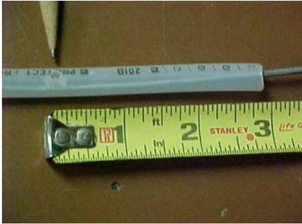
Now I measure 3" down from the top of the 3/8" plastic tubing and drilled a 1/8" hole. This hole is where I will attach my first rib.
