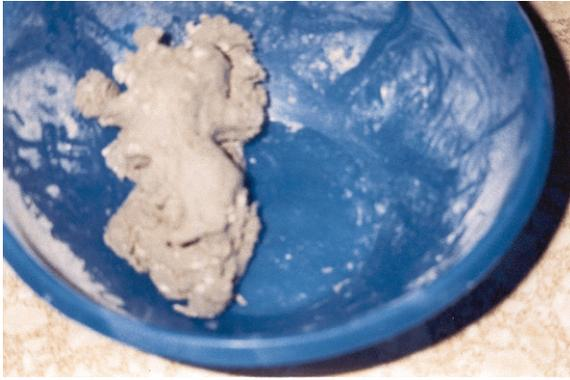
Mix desired amount of celclay with water .. mixture should feel like normal clay.. not too wet.. the wetter it is the longer it takes to dry so keep that in mind when mixing. Also keep a bowl of fresh water near by to keep your hands wet while applying.. this keeps the celclay from sticking to you and helps to smooth out any bumpy or rough parts.
