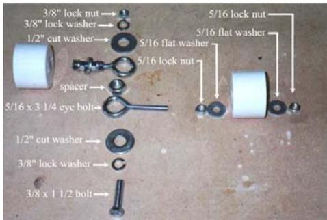
Before our dummy can begin to take shape, we will need to assemble all 12 of his joints. This will entail preparing the pipe cap fittings with the necessary 5/16" hole in the center of each. Also you need to assemble the joints and attach them to each cap. Here you can see how each section goes together.
