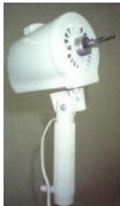
We are removing the motor cover so air can circulate around it for cooling and when we ultimately dress our dummy we will leave an opening at the top of the chest (through the neck) for the hot air to escape. Do these things and you should be as fortunate as I
