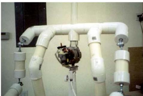
In the photo here you can get a really good idea of how our pose able dummy is constructed. As covered in the materials list, the PVC pipe you see is 1 1/2" schedule 40 and the joints are made up of a combination of the eye bolts, bolts, washers and lock nuts covered in our last section.
