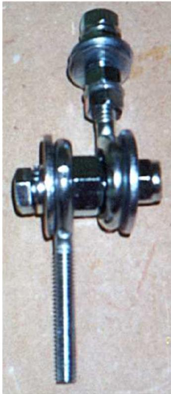
At the top of the blow up of the joint above shows two regular nuts on each side of two flat washers with a lock nut between each pair of nuts. My idea was to really lock the connection tight when attaching to the PVC cap.
