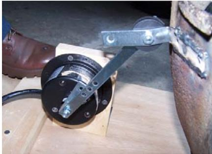
Everything is fastened to a nice sized chunk of plywood. I ordered two Mirror Ball motors off from Ebay, quite cheap! They are 5RPM and will hold up to 25 lbs. This one is turned sideways and screwed to a piece of 1 X 4, then used metal brackets to fasten that to the plywood.
