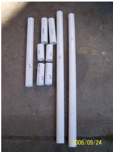
He's made of a simple PVC frame. Here you can see I have all the parts marked and cut. I used 1 1/4" PVC. All pieces are cut to what ever length you need for the size wanted.
