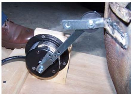
Everything is fastened to a nice sized chunk of plywood. I ordered two Mirror Ball motors off from Ebay, quite cheap! They are 5RPM and will hold up to 25 lbs. This one is turned sideways and screwed to a piece of 1 X 4, then used metal brackets to fasten that to the plywood.
