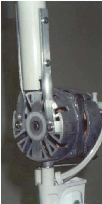
I cut a couple of sections of aluminum stock that was 1/8" x 1/2" x about 5" long apiece to attach to the motor housing into the threaded hole on each side of the motor shaft that the fan cage used to attach to. I bent an 80 degree turn a couple inches up on each, making sure that I bent one to the right, and one to the left so they would be able to cradle the 1" PVC pipe "neck" that I want to be centered directly above the pivot point of the motor.
