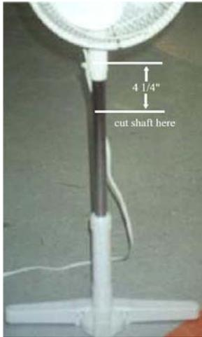
Next, remove the steel shaft (that came with the fan) that goes up inside the section of plastic pipe that the fan motor is attached to, cut this off at 4 1/4" long. Notice in the picture above the "cut shaft here" is shown with the top line at where the steel shaft begins once inside the motor mount. I use this photo here only to clarify what item needs to be cut down. The amount left sticking out of the motor mount that we will be inserting into our dummy's fitting will be about 2".
