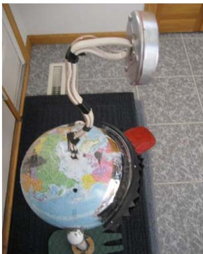
You'll notice the "eye" has some speaker wire attached to it. This is actually one of the battery operated ["pumpkin lights"](#) that changes from red to green to blue. I screwed this into the house wire stalk. I made my own battery adapter to replace the 3 AA batteries that normally run the eye. You can run it off batteries if you wish. Make sure you don't block access to the battery holders on the back of the light if you want to do this.
