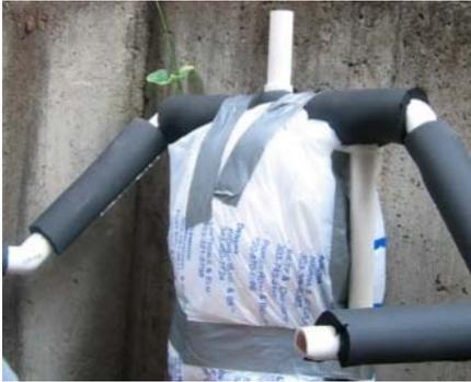
After the PVC pipes were assembled, we attached pipe insulation in various spots to simulate the muscles and shoulders of our frail, old friend.
