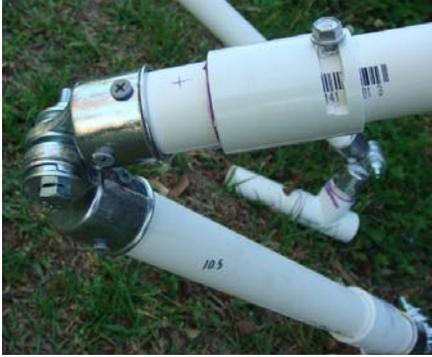
Here you can see the metal hinges and the PVC rotators
