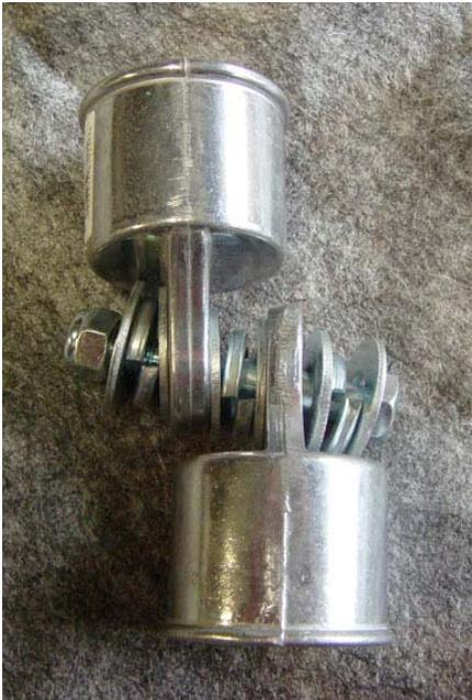
I used the same "spring tension" system to bolt the "bones" together and create working hinges / joints
