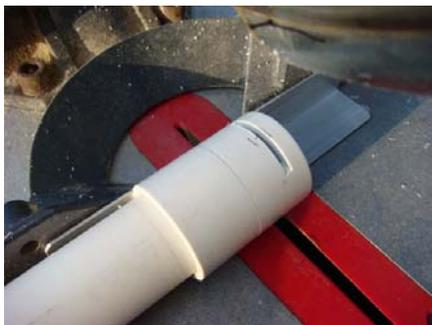
I used the miter saw to to carefully slice open a slot in the coupling, and a screw to hold the "bones" together.
