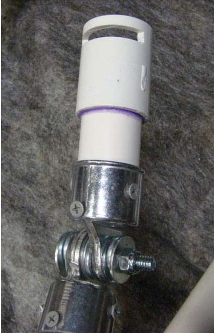
The coupling is only glued on the un-slotted side....the slotted side is dry fitted so that it can spin.
