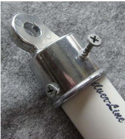
The metal fence caps are slightly larger than the PVC, so I used coated deck screws to hold them together.
