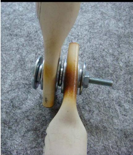
Just warm up the PVC with a propane torch and mashed between 2 steel plates.
