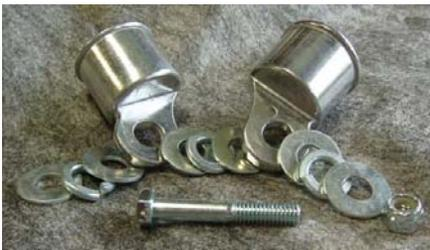
Here is the set-up for the hinge....flat washers and lock washers bolted through the eye holes with a lock nut on the end.
