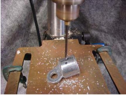
I used the drill press to add holes on all 4 sides
