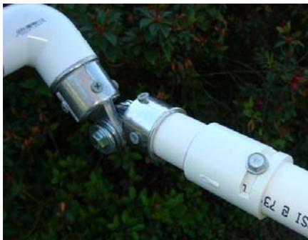
The pin and slot rotators are made with a 1' PVC coupling.
