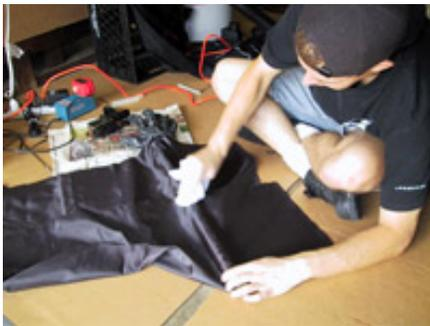
Hot glue is just that, hot. To press down the fabric into the glue we just used a plastic bag. Anything could be used; we just didn't want to touch it directly with our fingers.
