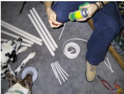
Here you can see all of the parts needed for the construction of the hands. The foam, PVC, tape, and wire all came to about 30 bucks.
