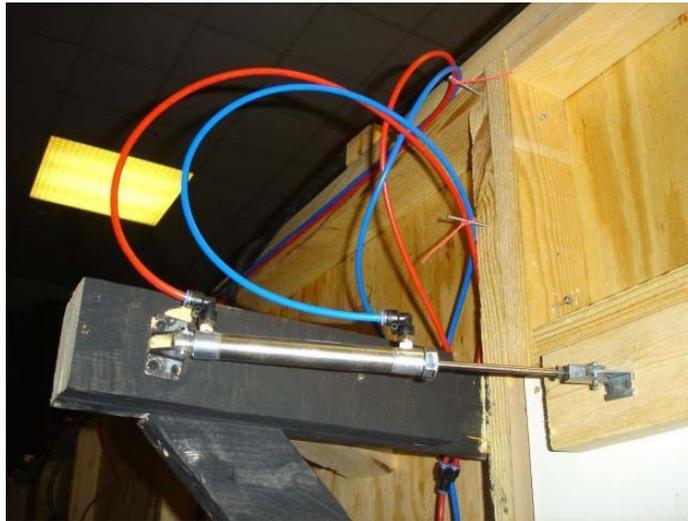
Above is a dual-acting cylinder. Can you see why? No spring involved, air pushes it back and forth. It will stay either extended or retracted until the solenoid is activated, then when activated, will reverse, and when deactivated, will return to it's previous state. Is this making sense? Good! If not, post some questions. Is this helpful?
