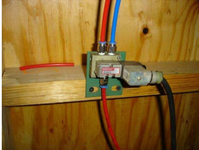
Do you see the little connectors I am using? Those are 'quick-connects' or 'instant-fittings', depending on where you buy them. I paid 63 cents each for those that go straight out from the solenoid. They are 1/8" NPT threads and adapt to 1/4" polyethylene tubing. The tubing costs \$7.50/100' roll.
