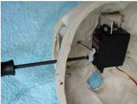
At some point, you're probably going to need to adjust the position of the servo horn on the servo. I recommend drilling a small hole in the side of the skull, as shown left, to accommodate a small Phillips screwdriver. Be careful when drilling the hole so as not to slip and drill out the center core of the servo (please don't ask me how I know about this).
