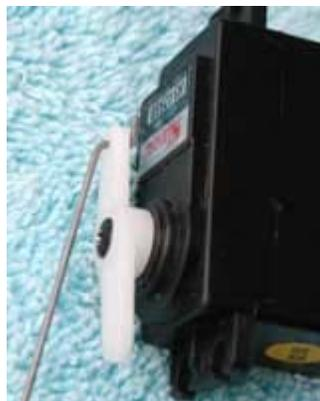
Next, using a pair of long nose pliers, create an offset bend, as shown left, in one end of a 6" piece of the music wire. Attach it to the outer hole in the servo horn as shown right.
