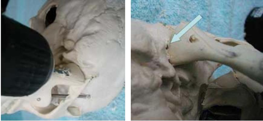
Bucky's jaw is held in place by a pair of springs. We need to install a permanent pivot for the jaw and also eliminate the springs because they are too much mechanical resistance for the servo. We'll use the cable ties as our pivot.
