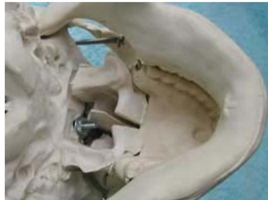
Using the #6 screw, nut and washer, mount the servo bracket in the Bucky skull. Tighten securely but don't over tighten as it might bend the bracket.
