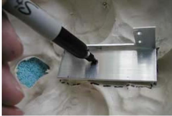
On the inside of the skull, right above the flat area shown above right, make a mark. Place the servo bracket where it will be mounted and transfer this mark to the bracket.
