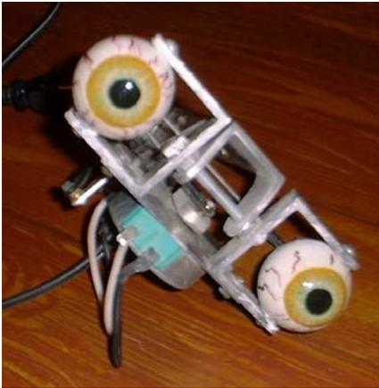
Near the center of this picture you can see the crank for the left/right motor
