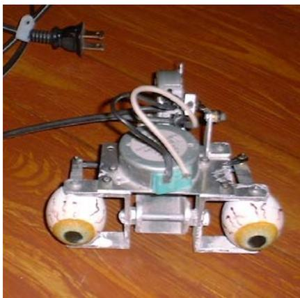
This front view shows the left/right motor mounted. You can also see the up/down link attachment.
