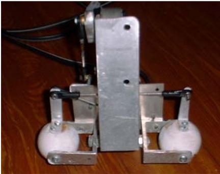
Bottom view showing main frame, eye mounts, and linkage for left/right movement. Control arms mounted on back of eyes are made from aluminum angle. L/R movement linkage works just like the steering in a car (except rack and pinion) the crank controls one side, a tie rod controls the other
