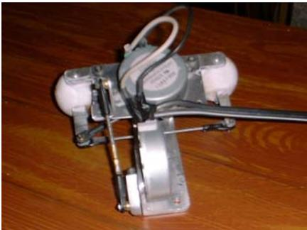
Top view with a better look at the up/down crank and the left/right motor mount.
