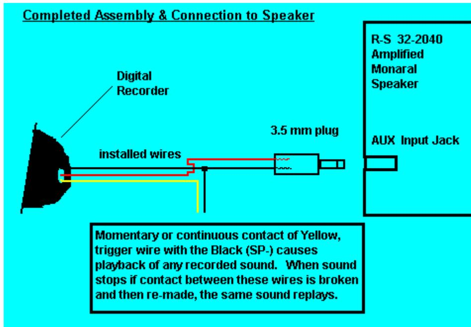
F) Attach a second Black wire to make a "T" connection as shown. This separate black wire will be used with the Yellow (trigger) wire to trigger the sound as explained in the diagram above. Also connect the Red and Black speaker wires to a standard 3.5 mm Plug.
