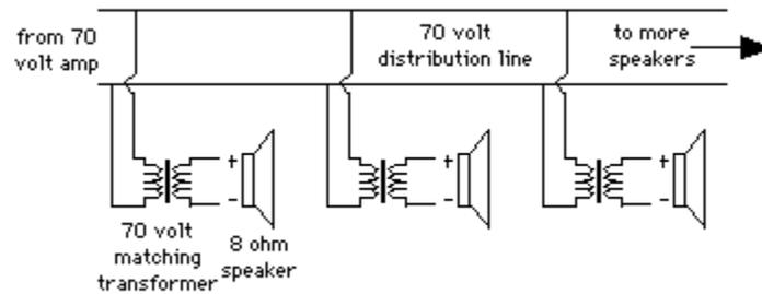
Each speaker has a transformer that 'taps' power from the distribution line, and converts it for use by the speaker. This method is extremely useful for very long wire runs. It keeps the cost of wire and speakers low - but adds the additional cost of the transformer. Unless you are using wire runs in excess of 100 feet, the 70-volt system may not be cost effective.
