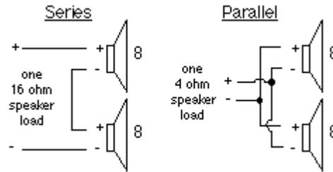
For series connections, always connect the (+) terminal on one speaker to the (-) terminal of the next speaker. For parallel connections, always connect (+) terminals together, and (-) terminals together. This keeps the speakers all moving together, delivering the maximum amount of sound possible.
