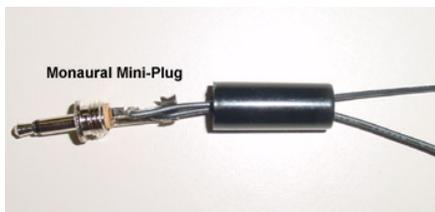
The other ends of the two wires from the mini-plug are soldered to the existing "solder mounds" of the two speaker wires. There is no polarity. That means: it doesn't matter which wire of the two goes to which solder mound. In the above photo the two black wires from the mini-plug are shown soldered to the same mounds as the two red wires from speaker.
