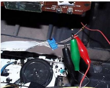
Here is a picture of how I probed wires into the CD player cable of the same boom box. The resistor you see here is merely being used as a piece of wire to reach inside the ribbon connector and has nothing to do with accessing the amplifier.
