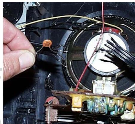
capacitor is just an option. Simply using your finger or a needle would work, but the capacitor makes it easier to hear the sound. When you find which wires make the noise you have found the right ones. You should be able to determine the left and right channels on a stereo unit. These are 2 of the 3 wires you will be tapping into.
