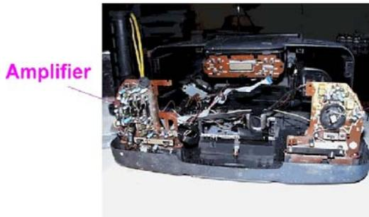
For our first way to make this old boombox into an amp, we will be using the part previously used by the radio.
