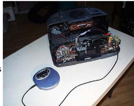
With the two units now connected with your test patch cord, turn on your audio source and press play. This test proved successful in using the cable that went to the amplifier from the radio. In the next picture we will show you how to use the other sources of your boombox if a radio isn't present or just unavailable.
