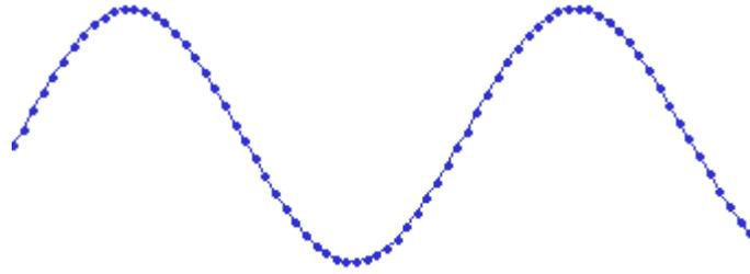
Each dot in the figure above represents one audio *sample*. There are two factors that determine the quality of a digital recording:
