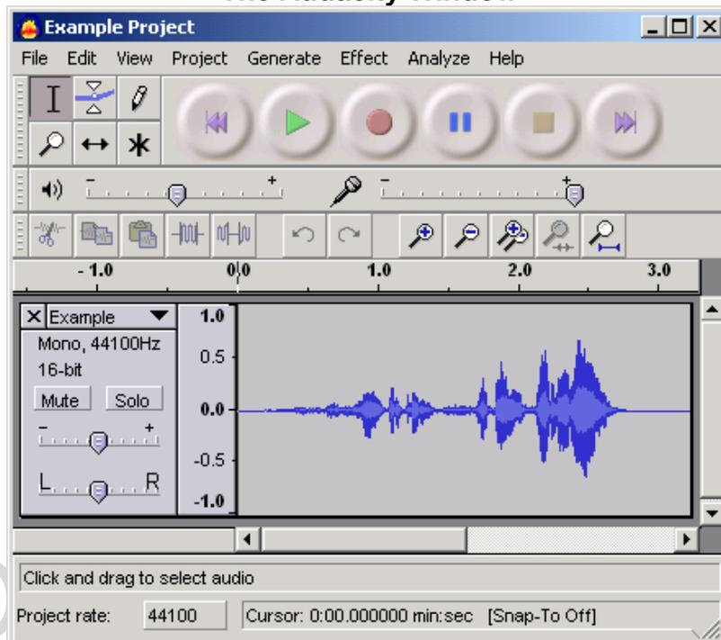
As you can see by the graphics above, the [time shift tool](#)
