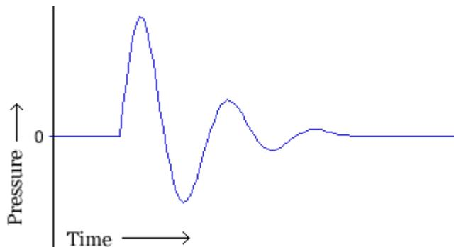
A hand clap is a short event that causes a single pressure wave that quickly dies out. The image above shows the waveform for a typical hand clap. In the waveform, the horizontal axis represents time, and the vertical axis is for pressure. The initial high pressure is followed by low pressure, but the oscillation quickly dies out.
