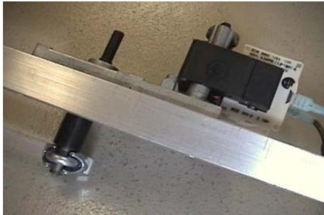
As you tighten down the nuts on this, keep the arm tilted downward as much as possible so the arm is slightly lower than parallel with the platform.
