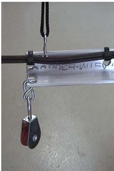
Here you can see that we have another S hook in the top hole, just barely above the power cord for suspending the back portion.
