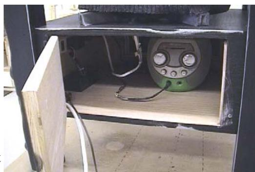
the analog cassette player altogether and replaced that with a Mimic Machine playback chip device. To amplify the sound from the playback device I used a small karaoke machine that you see here. Now rather than just talking all night, he merely plays back an 8 second clip as the TOTs pass by, triggered by remote control.
