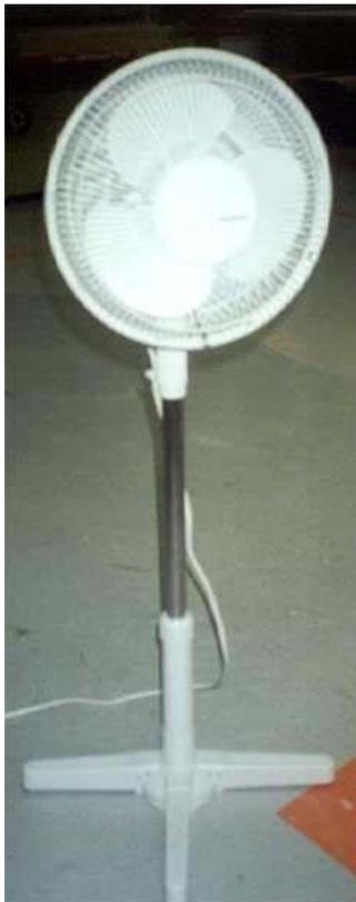
This is a standard 12" floor model Holmes stand fan that oscillates from side to side. This will be the mechanism to turn the head from side to side in a slow, natural movement of someone scanning the room. I start with this and simply remove the fan and fan cage. Cut off the shaft that sticks out the front that used to have the fan attached.
