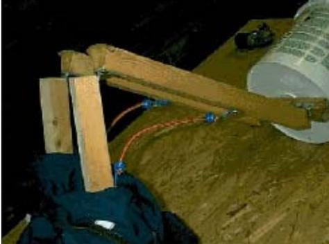
Using the strap hinges, attach the lower legs to the upper legs placing the hinges on the reverse side as the 'T' hinges (knee joints).
