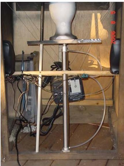
You can also see the 1x4 mounted onto the top of the cylinder, to which I attached the foam head (wire wrapped over it and secured to staples under the board; a strip of duct tape under and on top of the wire protects the foam head). Also note the thin PVC tube I mounted to the left of the cylinder; it is secured at the bottom and provides a "guide" so when the head/platform raises and lowers, it won't twist or turn to either side.
