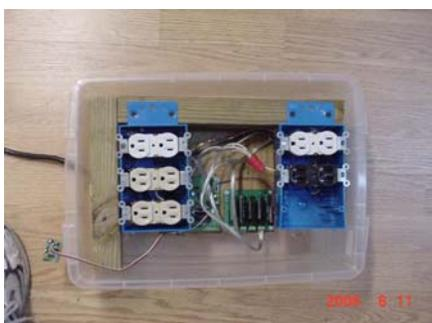
Here's the whole assembly tucked inside the plastic storage bin. The last picture is taken after I placed faceplates over the receptacles and labeled them.
