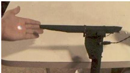
The beam emitter is a red "super bright" LED on the end of a cylinder which slides inside a tube. The tube has a 1" plastic lens mounted in one end. The cylinder slides in and out to focus the beam. The end of the tube is cut at an angle to form a hood which hides the glare of the light from eye level. At 25 feet, the beam spreads out to about a meter in diameter, but it's still bright
