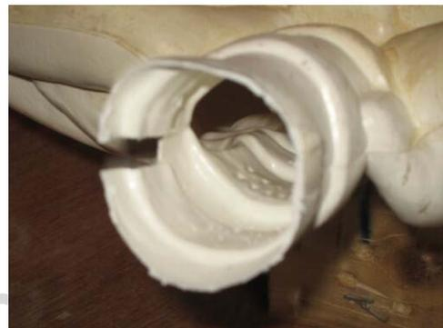
With standard HiTEC servos the neck slit should be on the blucky's left side, this may not be true of all servos so you should determine this before hand. Once the cuts are made force the servo into the neck with the connection wires in the slit until the servo mounts are flush with the top of the neck. Use a zip tie or two to hold the servo in place (Figure 7)
