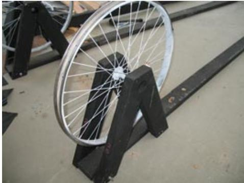
When the three hoops are joined together, they'll rest on three pairs of bicycle wheels. Of those six wheels, five are free spinning (like the one shown right) and the sixth is driven by a motor which rotates the overall tunnel.
