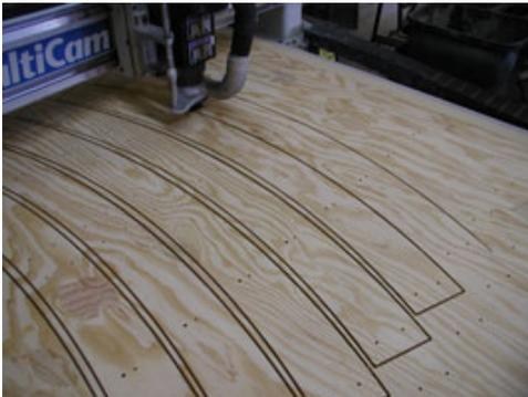
The individual pieces are cut from 1/2" plywood using a CNC router (thanks Jim). The accuracy of this device is absolutely amazing. If you're interested in getting your own set of hoops made, you can [contact Jim](#). I think he charges about \$250-\$300 plus shipping for a set of three hoops.
