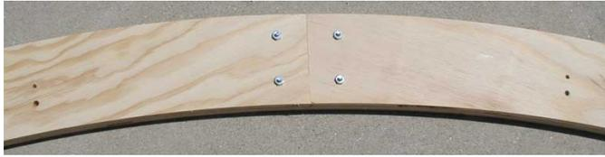
The joints fit together perfectly to form the complete circle. Note that I'm now using "T" nuts instead of loose nuts as shown in the above picture.
