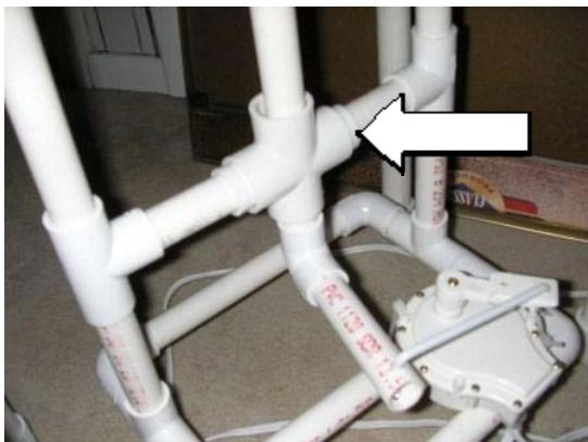
Here you can see the placement of the 1/2" to 3/4" bushings on the lower 4 way tee.
