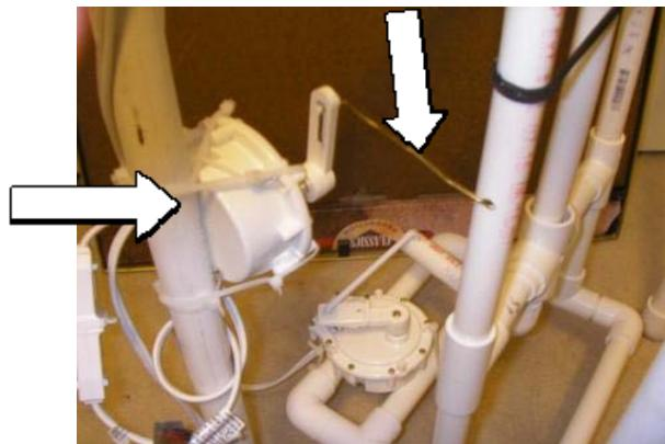
This arrow show a short section of coat hanger used as part of the crank. I just drilled a hole thru the PVC and bent the coat hanger so it would not fall out.
