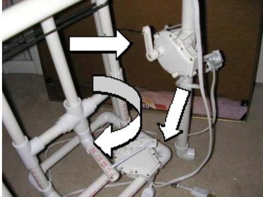
This shows both motor mount locations. The lower motor is attached to the swinging inner frame. In fact, the base of the swinging unit is built just to have a place to attach the motor.
