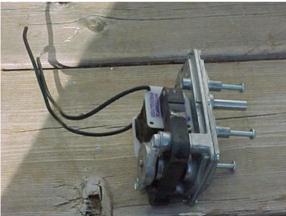
We used a Dayton 4RPM AC Gearmotor, item 3M098, that my husband picked up at Grainger for \$34 ([click here](#) for instructions using a rotisserie motor). We mounted it on its side to a small sheet of wood and then attached a block of wood to this as a base. This base we screwed into the bottom of the tombstone box. This keeps the motor stable and secure. Make sure you don't screw the motor to the wood sheet too tight or the motor will bind up and not spin.
