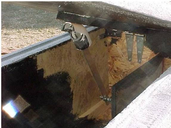
A view of how the crank works. The elbow PVC is mainly used as a device to hold the aluminum stock up. The stock isn't glued or screwed in - it's just set inside the PVC pipe. When plugged in the motor turns the shaft which rotates the L bracket. The aluminum stock rises and falls. The stock, which is nested inside the elbow pipe that is attached to the lid, lifts and lowers the lid.
