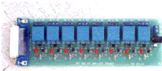
This relay, when attached to a computer running a very basic program, can be used to trigger multiple actions for any haunt. A computer program sends signals to the board triggering the eight (8) relays. The signal will either open or close each relay. A red LED tells you if the relay is energized. Each relay can be equipped to send out any voltage you wish. You route a power input voltage wire to the inlet screw on a relay and you control the output by firing the relay.
