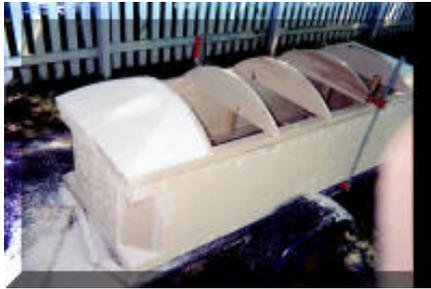
I carve the styrofoam with a hand saw, 3" belt sander and a really big file that I have. I used this foam on the ends so I could angle the short ends towards the center. (open the photo to see). This also is an addition that I felt just added that "BANG" to the looks of the final product.
