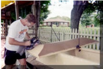
We covered the lid with a brown "peg-board" material that is the same as the boards you get to hang peg-board hooks on but it doesn't have holes in it and is only \$5. I used this board because it is flexible. Luan is too rigid to bend over the the arch. I glued the end wood pieces to the carved foam. The 3" belt sander is great for shaping the wood (wood putty is effective also)
