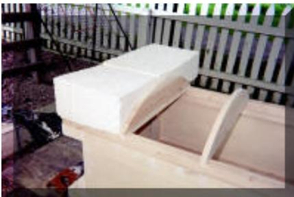
Next came the lid...Build a square frame from the 1 1/2" framing lumber that is the same size as the top rim of the coffin body. Now, fabricate "arches" from some 3/4" x 6" or 2" x 6" lumber. The arches give the lid a unique and realistic look.
