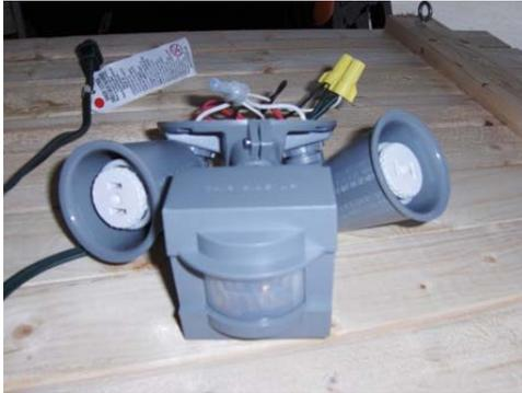
Step 5- Wire the motion sensor by adding an extension cord. It is really easy to wire up.
