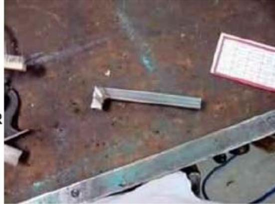
Aluminum Shaft Reinforced by Short  $\frac{3}{4}$  in Pieces and Bolts
