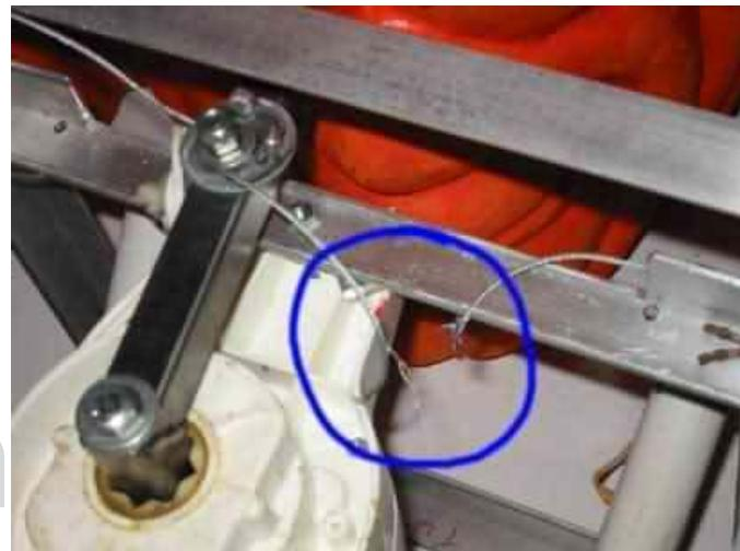
I found that the aluminum cables I had been using actually shredded! I was not expecting this since there was no sign of damage earlier. For this reason I am promoting the use of nylon rope, I have yet to test it extensively, but I believe that it will work just fine.
