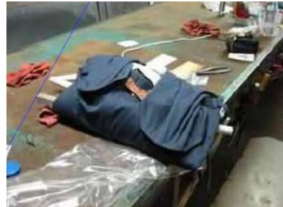
Unbolt the two bars that attach the motor to the frame and put the nuts and bolts in a plastic baggie. Loosen the 8 bolts that attach the front and back of the frame together and collapse the frame, keeping the motor sandwiched between. Stick the plastic baggie in a pants pocket, flank the motor with the legs, and wrap the pants around the frame and secure with wire, here is a picture of how small the prop can be collapsed down to.
