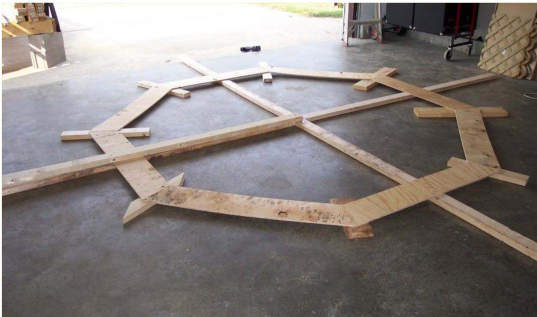
You can see the first layer on supports, and an arm that the router will mount to.
