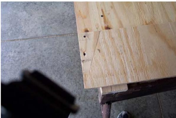
And here is the end that held the piece we were cutting. We used some scrap from cutting the angles to make a holder for each board that we could quickly place in the jig.
