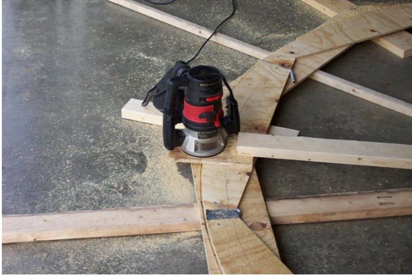
Here is a shot during cutting. This method would have worked great if the router bit was 1/2" longer! It was just short, and wouldn't cut both layers at once. We made the mistake of trying to flip the ring over, which didn't work. We ended up with a ring that had two cuts that did not line up.
