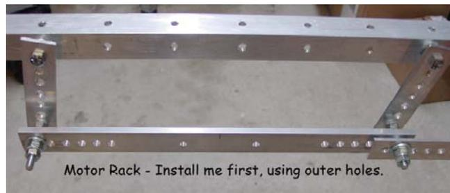
Connect the central pair of these little crank-like levers with the thick motor mount rack. Install it as close to the inside as possible. You want, in other words, for the motor mount bracket (rack) to be as close to the big parallelogram rack member as possible, to help with an upcoming clearance issue.
