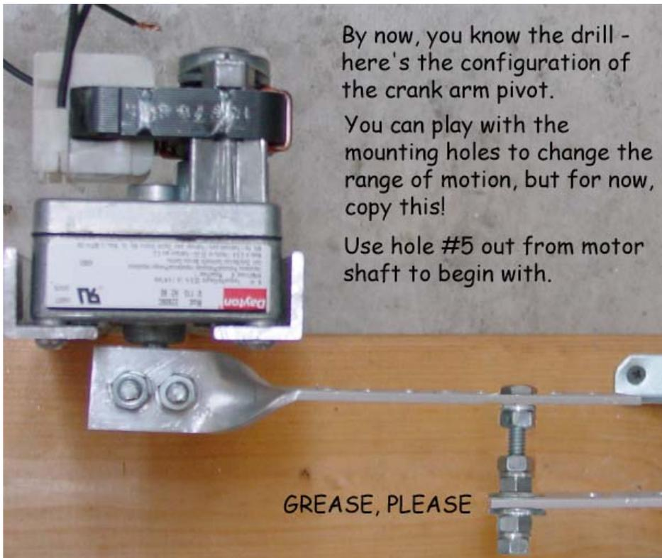
By now, you know the drill - here's the configuration of the crank arm pivot.
