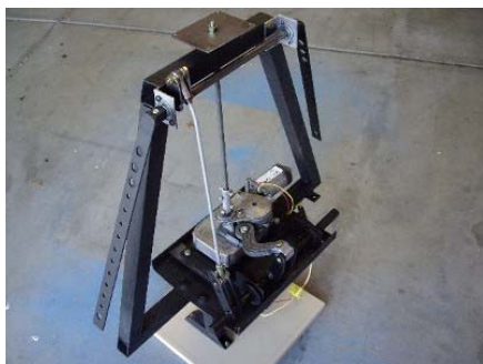
In the frame with linkages to arms and head pivot mount
