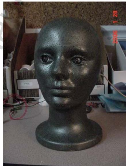
Worked out a few bugs in the PROP1/BS1 stamp code and now have that working pretty well. The PIR gets tripped, the PROP1 delays 15 seconds then turns the head around (via servo), lights the eyes up, and triggers the sound module. 20 seconds later the head turns back around and the eyes go out, and the PROP1 pauses for 40 seconds to ensure it can't be re-tripped right away.
