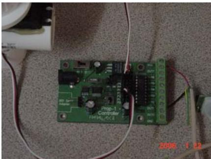
With a servo, and the other linked effects I wanted to trigger, it came time to consider the "brains" of this prop. For this I picked up a PROP1 board from Parallax.
