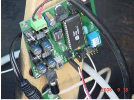
The solenoid on the bottom is what switches the airflow in the box-pusher cylinder, from open (out) to closed (retracted). The AP-8 is a mono sound device; we located a good sound clip of dog barking, and downloaded it onto the card. The card has a built-in amplifier which will power the 4-ohm external rock-speaker (seen above) LOUDLY.
