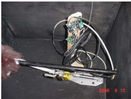
The end result is that the cylinder acts as a lever, moving the long PVC pipe forward and out the front of the doghouse when triggered. When it retracts, the pole gets slid backward, staying level thanks to the hole in the back which it slides out of.
