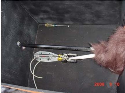
Here's where we started fitting all the mechanisms into the doghouse. The box pusher has a PVC pipe bolted to it, which in turn is bolted to a second long PVC pipe which extends forward a few inches (to hold the head) and straight back through a hole in the back of the doghouse.
