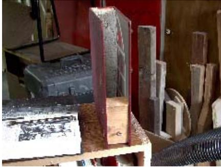
I wanted to test my idea by animating one book first so I started out by cutting almost all the way through a piece of PVC with my miter saw but stopped with about an inch left attached. I then used a piece of coat hanger to manufacture a push rod and soldered it so it wouldn't catch as the cam pivoted.
