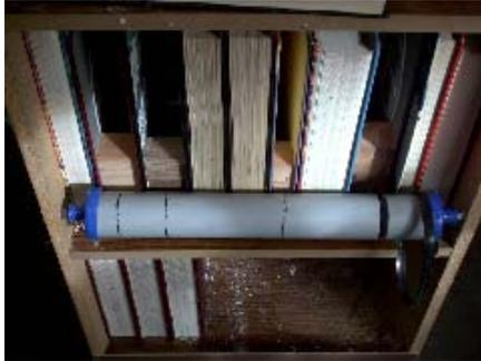
I manufactured push rods to match the others, attached them to the PVC and soldered them. I then attached them to the eye screws on the books and mounted the whole works back in the bookshelf. I had an old blender motor that I was able to mount underneath and attach the belt to.
