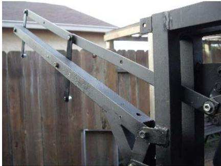
Link arms are attached to the bell cranks which Bluckies are mounted on. End result is that the Bluckies "swing" back and forth.
