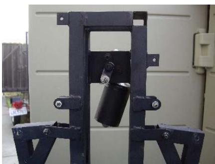
The crank arm of the wiper motor can be seen here.
