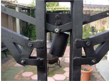
Limbs in place and link rods attached to crank. Rotation of the crank produces a back and forth movement.
