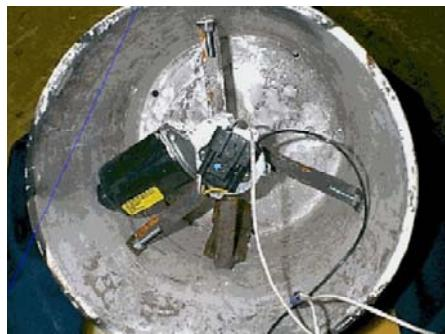
First you must start by measuring the inside diameter of your plastic pail and draw a circle as a layout. Place your motor with the shaft dead center of the circle. Measure the distance from the center of the motor shaft to the circle and subtract 1/2". You will need to either extend, or make a new crank arm with your counter weight at the end. This weight can be of practically anything that can be permanently attached to the end of the crank arm.
