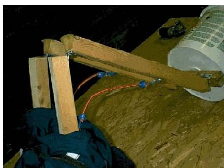
Using the strap hinges, attach the lower legs to the upper legs placing the hinges on the reverse side as the 'T' hinges (knee joints). You may want to glue small pieces of foam rubber to both the knee and hip joints to reduce banging when operating. With fender washers and drywall screws, install the bungee cords from the upper to the lower leg pieces as shown on the right. These can mount practically anywhere on the leg. I suggest that you don't mount the bungees exactly the same on both legs.
