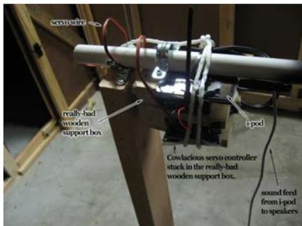
At the other end of the 5' long PVC pipe, I attached a make-shift wooden box to hold the servo controller (I bought it from [Cowlacious](#) rather than making it myself. I made sure the box hung down below the pipe when the skull was oriented upright. This way the skull would naturally stand straight up. Also shown in the picture is the wooden support and a metal support bracket to hold the assembly up when I am not moving the head (more on that later).
