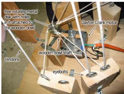
The Flying Crank Ghost (FCG) mechanism is very versatile. I use it in a different manner for the crystal ball. It is simply a slowly rotating shaft that pulls your strings in a way that makes your prop look alive.
