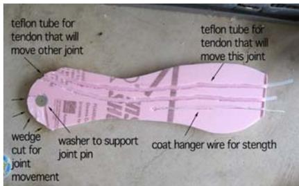
You must make three measurements before you can make the last piece. You need to align the washer to the middle joint just like you did with the claw. But now, you have two tendons to align. The inner tube will hold the tendon that runs all the way to the claw. The other tube will hold the tendon that will move the center bone. The rest is just a duplicate of what you just did.
