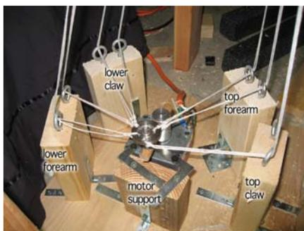
There are lots of tutorials on the Flying Crank Ghost so I am not going to go into that much detail in the mechanism itself. Here are the basics. I have a Dayton Crank motor that rotates at 6 rpm. You do need a motor with some reasonable torque to make this work. I attached a 4" wooden dowel as the shaft. I surrounded the motor with four blocks of wood and put 2 eyebolts in the top of each. The tendons ran through these eyebolts and to the free-rotating metal disk attached to the dowel.
