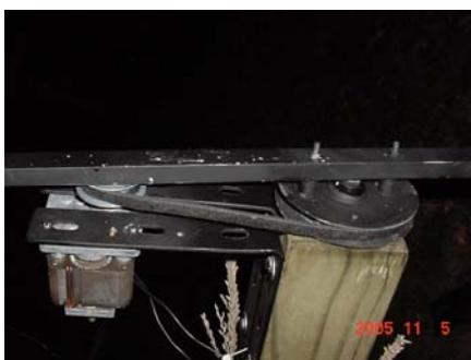
I mounted a small pulley wheel mounted onto the motor shaft (size of the pulley wheel will depend on the speed of your motor, and how fast you want your witches to fly around). My motor is a 13 RPM high-torque motor. An automotive belt from the local hardware store links the two pulleys. Once you get the motor lined up, drill holes in the angle irons to attach the motor.
