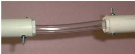
To create the flexible elbow and forearm, glue the bushing into the ends of the forearm and upper arm (You will need to sand the inner part of the tube with a Dremel tool and a barrel sander) and once dry, drill a hole large enough to accommodate the machine screws. Now connect all the parts with the screws
