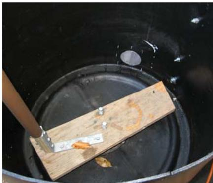
A simple 4" "L" bracket was mounted to a board mounted to the pulley system to hold the pole in place. The pole is held in place by a 3/4 x 3/4 inch board 3' in length. The PVC pole slid right over it.
