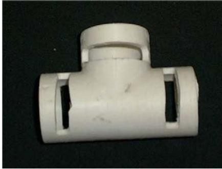
Now that everything is cut to length, take one of the T joints and the cross piece and cut two slots out of each side using your Dremel tool and a cut off wheel. Refer to the pic here to get the idea.
