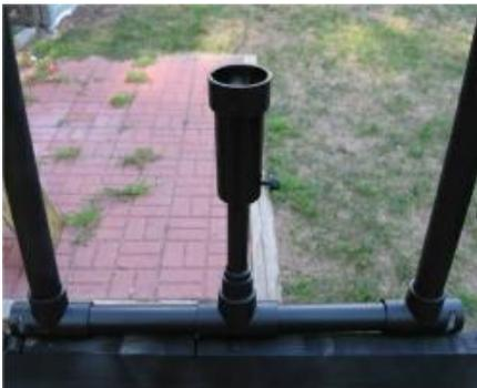
This is the fan's mounting piece. It fits right onto the 1/2" PVC and has its own set screw to secure it. Now just mount the fan into this piece, and it to has it's own set screw to hold it in place.
