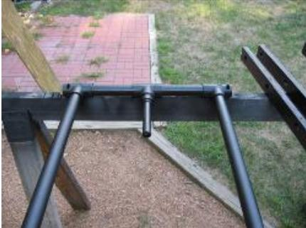
This may be hard to see but this is the hip/pelvis area as assembled. In the center there is a two inch long piece of 1" PVC glued in first. In to that is one of those bushings that you have again removed that ridge from.
