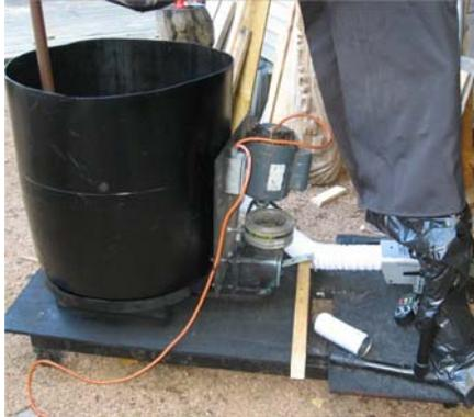
Here You can see the rough in of the whole mounting system and the trolley. I also sprayed the power cord black so it would fade into the background. The PVC frame of the witch is mounted by two 1" C clamps screwed on to the wood base. Below is four views of the finished project. I actually oiled the pivot points so aid in movement and to quiet them some. (They squeaked loudly.) I used green coated floral wire to tie the hands together on the pole to help them stay in place.
