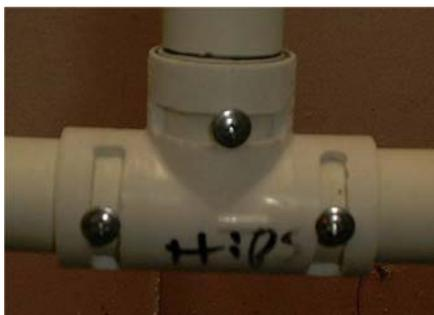
Add the leg sections and the 90 degree hip section as well. Do not glue the torso section, these will be screwed in to place using the wafer head screws. (Pic #7 and #8)
