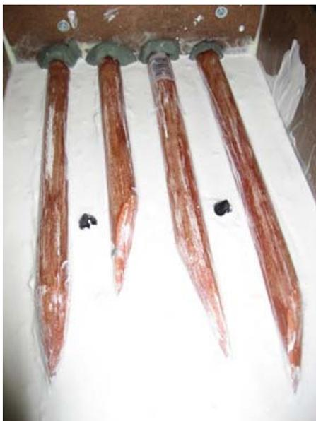
Believe it or not, this was the toughest part. I recently figured out how to make latex molds so I figured this would be easy. I carved four spikes from 1" wooden dowels and made a latex mold. I then got some 2-part 8lbs polyurethane flexible foam, mixed and poured.
