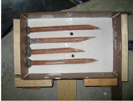
This approach worked fine when I was making skulls with ridged foam. The problem I discovered is that flexible foam is really hard to get out a a mold. It sticks more than the ridged foam and, since it flexes, there is nothing to push against. After ripping apart two of them, I just cut the others out, thus destroying the mold. I also found that this stuff is almost impossible to sand, so get the shape right or plan on using scissors.
