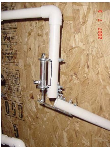
The Bimba cylinder used only has a 1" movement (which is all I needed to move the arm from a 90-degree position, to a slightly dropped position when Private Waltrip lights the cannon). The elbow is a simple hinge screwed into the PVC; the cylinder providing the motion is mounted behind the arm and held in place by two eye bolts that I found that just happened to be the right size to hold the cylinder in place.
